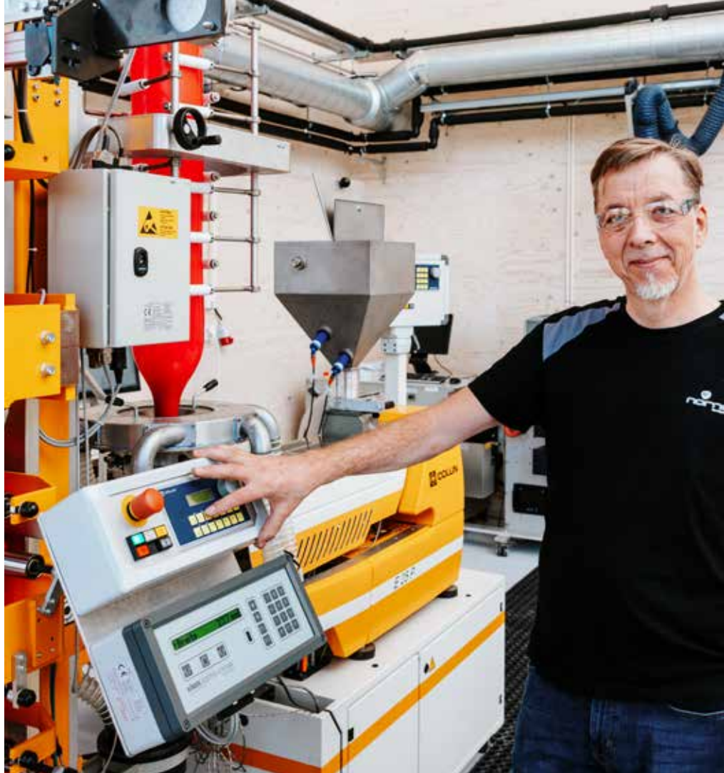
Norner has several pilot lines for blown and cast film extrusion up to 7 layer. This is a very flexible set up for product development.
