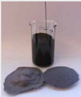
ReSiTec silicon kerf from diamond wire sawing
