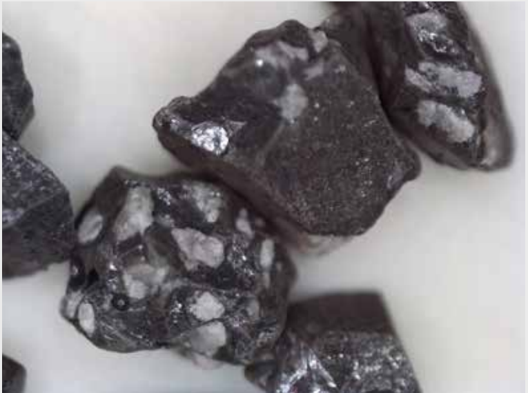
Particles from sculls 0-6 mm, a mix of slag and silicon. The white particles are probably undissolved silver sand.
