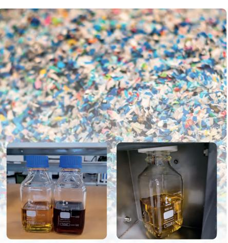
Figure 2 Photos of fluffy plastic waste and resulting pyoil
