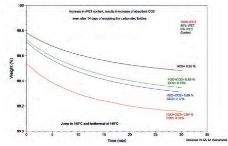
Figure 2 TGA isothermal analysis at 140°C
