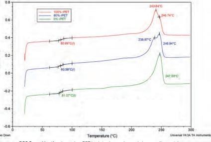
Figure 1 Effect of rPET amount on the crystallisation behaviour and crystal morphology of PET using DSC.
