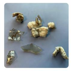
Figure 3 (Left) Popping and (right) lump formation (along with degradation) due to a combination of CO<sub>2</sub> absorption and slow cold crystallization due to the presence of high amounts of 100% recycled PET.
